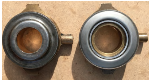
Fig. 2. Original clutch thrust assembly (left), new sealed thrust bearing (right).
