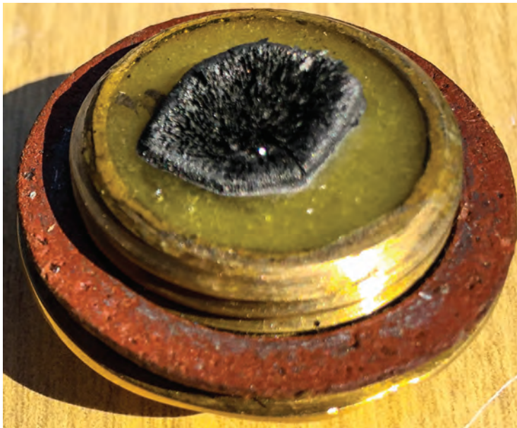
Fig. 9. The gearbox magnetic debris collector.
