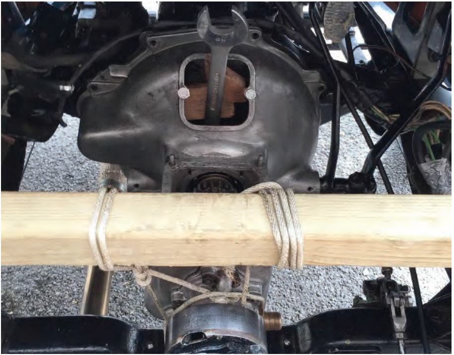
Fig. 4. Separating the gearbox from the engine.
