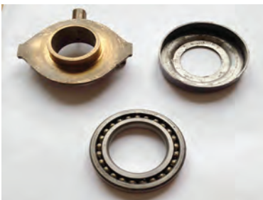
Fig. 1. The original clutch thrust 'open' bearing assembly.
