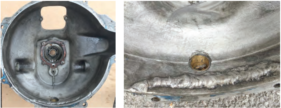
Fig. 3. Aluminium bell housing weld repair at base.
